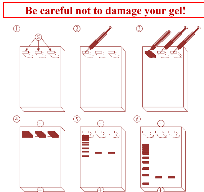
Figure 2 - 2.2 – Schematic representation of the electrophoresis process. S – slots/wells.
