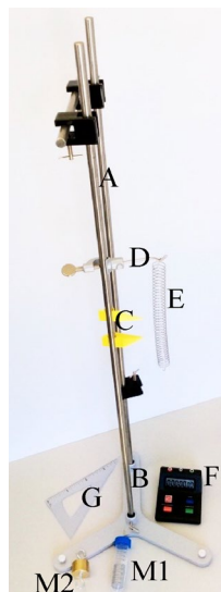
Figure 2 – 2 – Equipment used in 2 - 1.1: standing structure (A) mounted on a standing base (B), pointer pair (C), clamp with hook (D), spring (E), plastic tube with a suspending thread containing a pair of bar magnets (M1), brass mass (M2), stop watch (F) and square ruler (G).
